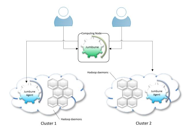
Multiple users running single deployments of Jumbune can use or share the different clusters, either to monitor it whilst running a debugging or profiling job or run validations on the HDFS data.
