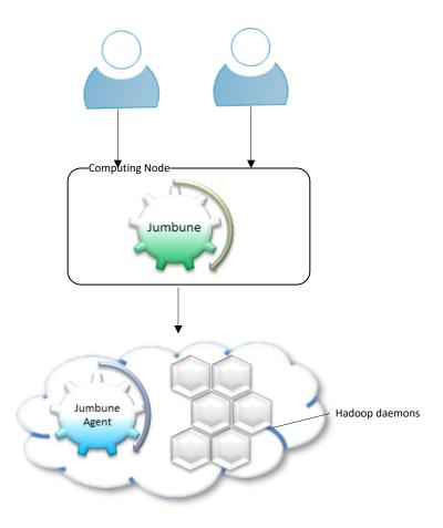
Jumbune's **Debugger** and **Job Profiler** can be used on the **staging environment** to ensure that there are no performance bottlenecks or flaws in the job when it comes to realistic data. The QA and dev team could use the same deployment of Jumbune to access the cluster and perform various functions on it as described in the previous sections.
