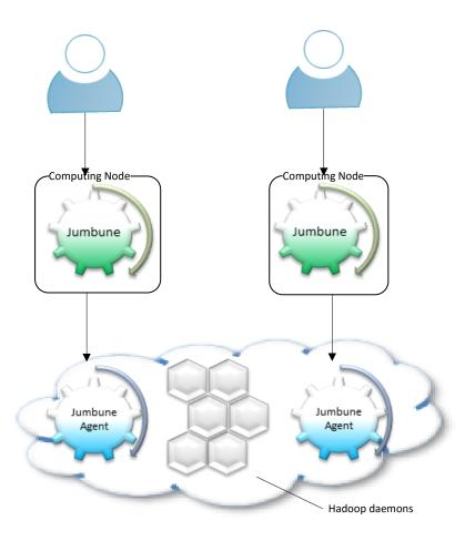
Multiple users running multiple deployments of Jumbune can use the same cluster, either to monitor it whilst running a debugging or profiling job or run validations on the HDFS data. Performance engineers or cluster administrators could keep a watch on the various cluster metrics using the **cluster monitoring tool**.
