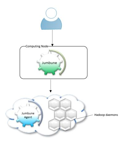
This scenario would be useful in the QA environment, where a quality engineer could connect to an agent running on Hadoop cluster and perform various levels of testing.
